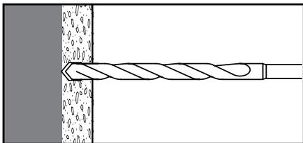
1.) Drill the proper size hole into the cavity of the base material.
