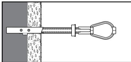
2.) Position the wing parallel to the plastic legs and slide the anchor through the drilled hole into the hollow cavity.
